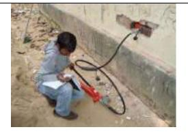
Photo 29-30: Test set up for In-situ Shear test
