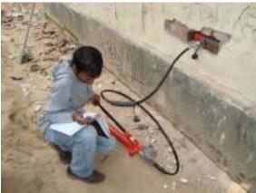
Fig 3. Test Set up for In-Situ Shear Test
