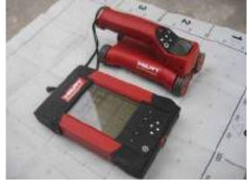
Photo 27: Use of rebar detector for verification of reinforcement details
